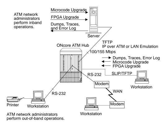
Figure 6-1. Upgrade Operations for ATM Microcode
